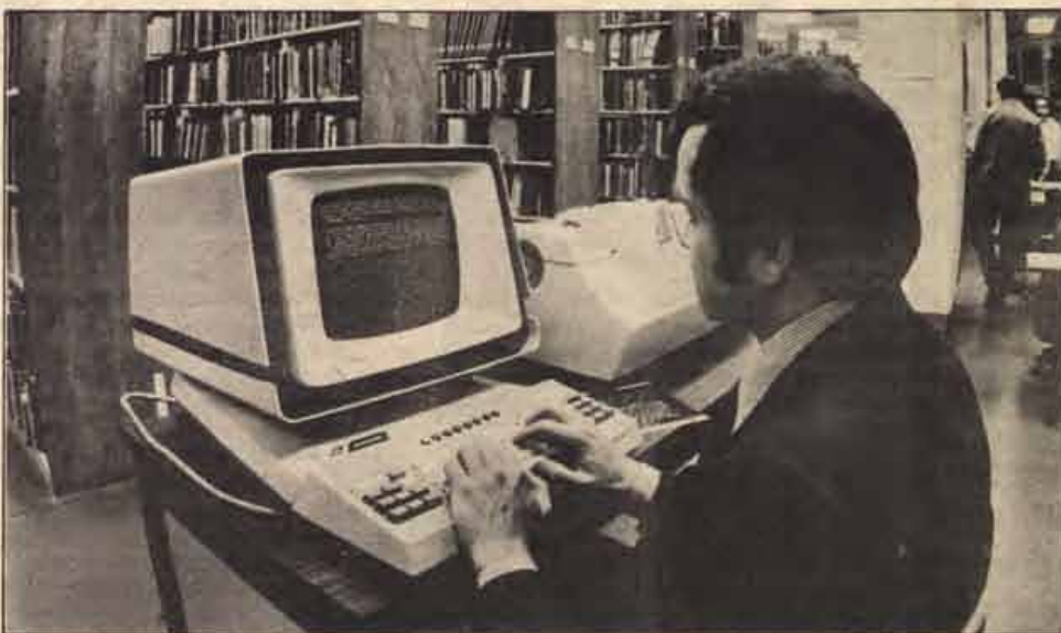
A CRT (Cathode Ray Tube) Terminal. There are 60 such instruments throughout The Times building.
